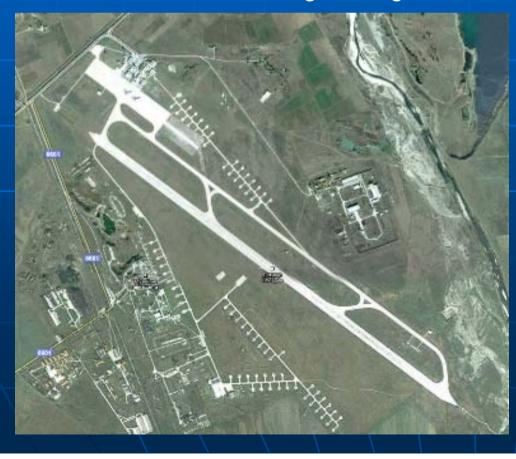
The size of the apron is 800 by 111 m. Most of the apron, 85 %, has concrete pavement, and 15 % are paved with asphalt. The apron has 13 aircraft berths, of which 6 are designed for type "C" aircraft, and 7 – for type "D" aircraft. The apron pavement is in a good condition. The airport is equipped with an instrument landing system (ILS) for Runway 30; landing at Runway 12 is subject to visual flights rules. The system used is D-3.
