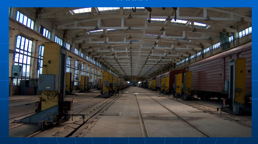
Bogie replacement yard – 2 multi-purpose tracks with 12 stations each. The yard's capacity allows to replace the undercarriages of 280 railway cars in 24 hours.
