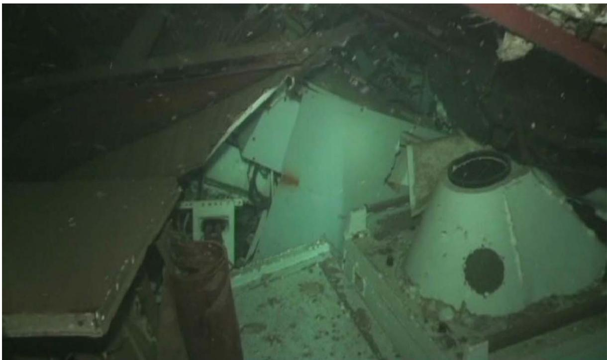
The navigation bridge is heavily bended down in the middle. Starboard side wing door of the bridge is opened and the port side wing one is closed.
