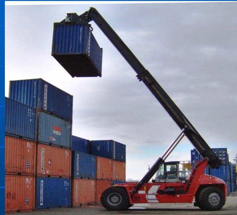
The terminal is equipped with a new latest-generation container loader model RDF450-60S5X, manufactured in Sweden by “Kalmar Industries”. The terminal allows stacking of full 42-tonne containers up to a height of 5 m.
