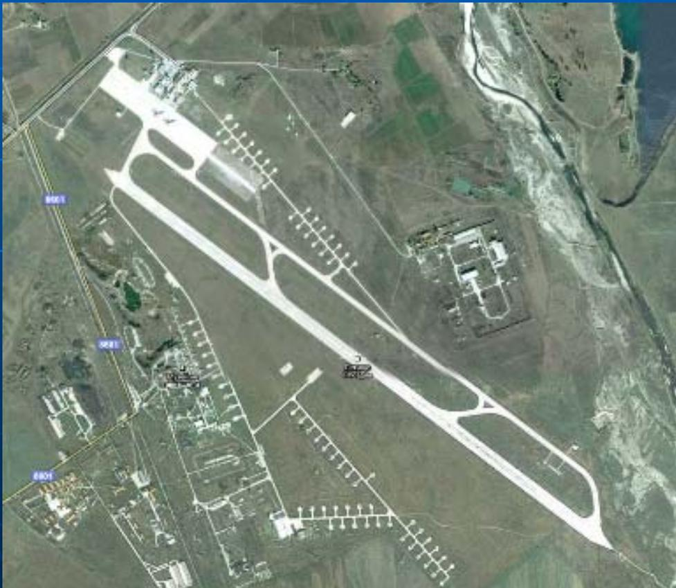
The size of the apron is 800 by 111 m. Most of the apron, 85 %, has concrete pavement, and 15 % are paved with asphalt. The apron has 13 aircraft berths, of which 6 are designed for type “C” aircraft, and 7 – for type “D” aircraft. The apron pavement is in a good condition. The airport is equipped with an instrument landing system (ILS) for Runway 30; landing at Runway 12 is subject to visual flights rules. The system used is D-3.
