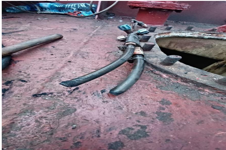
Fig.7. The used gas cutter, after removing from the tank
