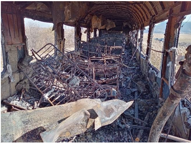
Fig. 1.5. Condition of the internal part of passenger coach № 50522974242-2 after the fire.
