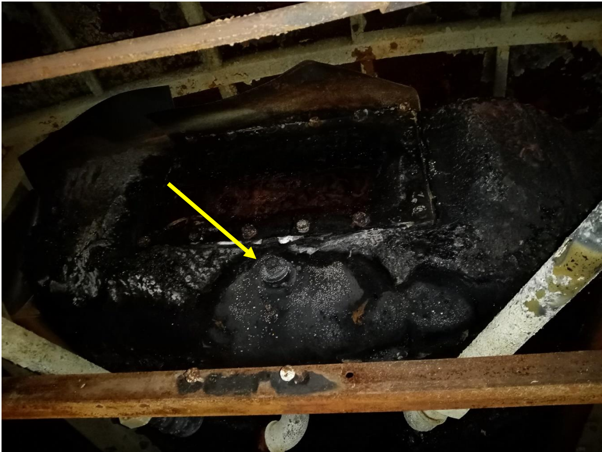
Fig. 4.19. The arrow shows the outlet in which the heater is installed. In the specific case the outlet is closed with plug, because no heater was installed.
