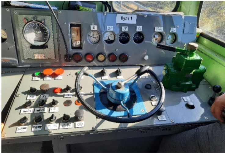
Fig. 4.3. Layout of the facilities and apparatuses of panel № 1 of locomotive № 98522051522-7.
