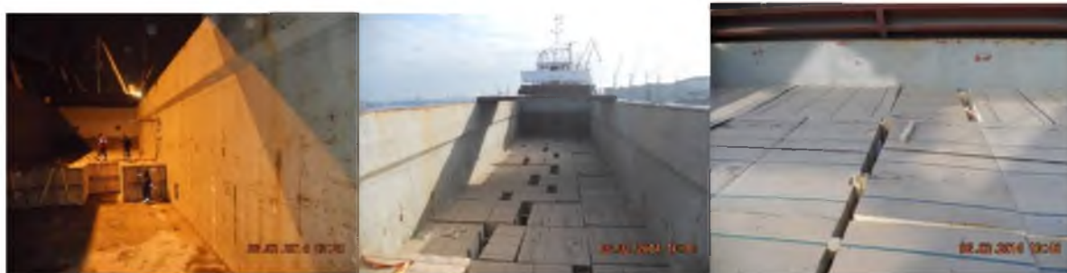
Fig. 2. Stages of loading and consolidation of the cargo in the hold.
