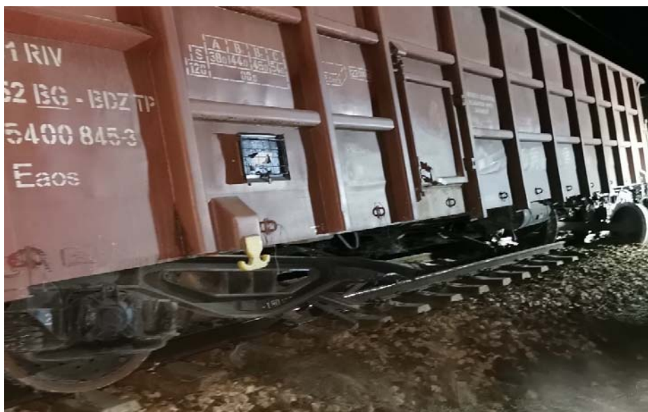
Fig. 1.1. Derailed the first bogie of wagon № 31525400845-3 along Shivachevo – Tvarditsa interstation
