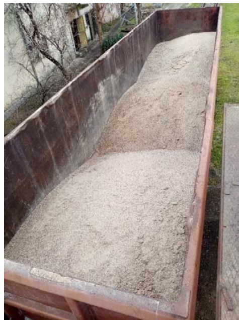
Fig. 5.1. Distribution of the load in 16th wagon № 31525400845-3
