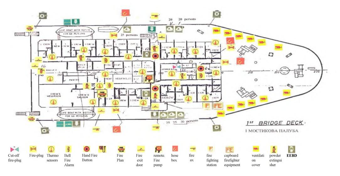
**Fig. 4** 1<sup>st</sup> bridge deck fire plan
