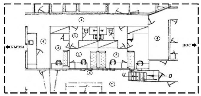
**Fig.** 7 A part of the cabin plan on the first bridge deck s/b side 1,2,3 - Cabin of the seamen/messmen / 1 and 2 - Bedrooms, 3 - Antechamber; 4 - Corridor; 5 - Cook's cabin; 6 - Place of hot works; 7 - Deck.
