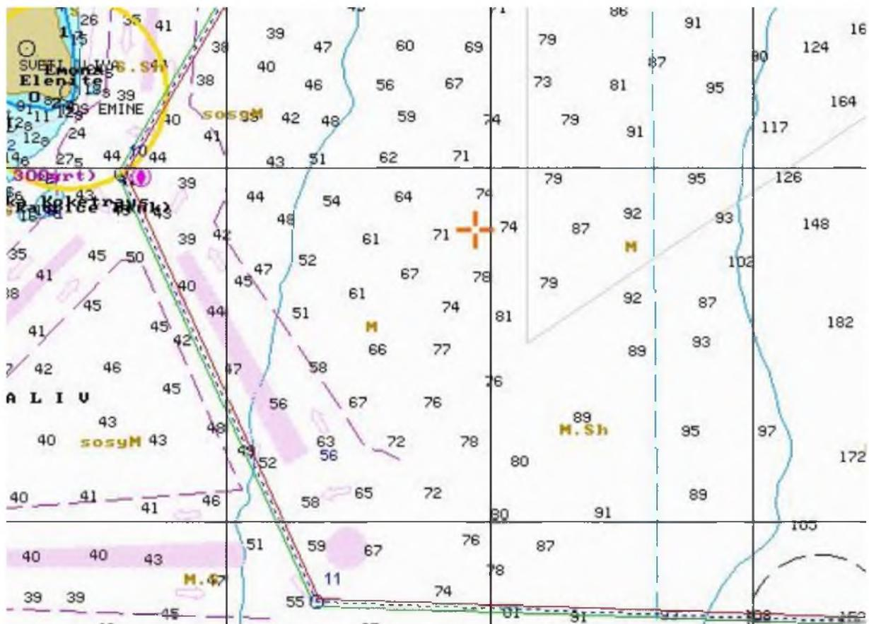
Planned route of the m/v „St. Catrien” – entering and leaving the Traffic Separation Scheme southeast of Cape Emine. Data from the vessel’s ECDIS.
