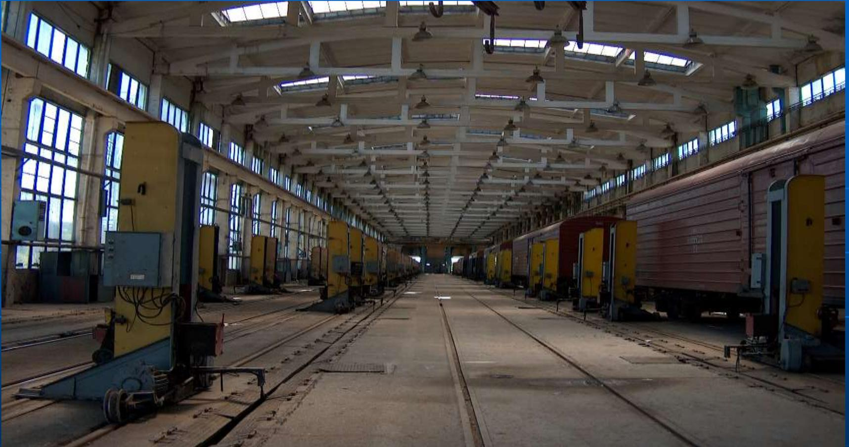
**Bogie replacement yard – 2 multi-purpose tracks with 12 stations each. The yard's capacity allows to replace the undercarriages of 280 railway cars in 24 hours.**
