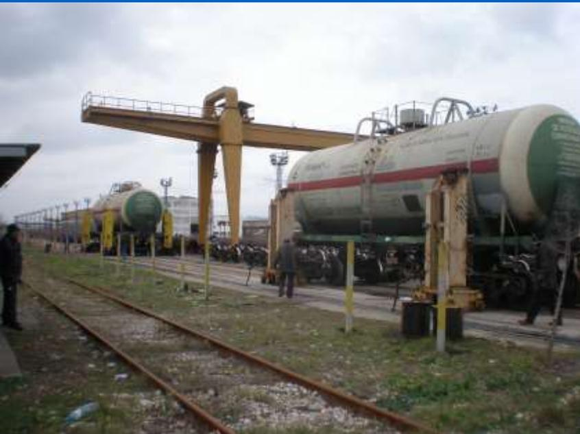
Track for replacing the undercarriage of railway cars with hazardous cargo – with standard-gauge tracks, and two stations fitted with explosion-proof jacks. The yard can handle up to 20 railway cars in 24 hours.
