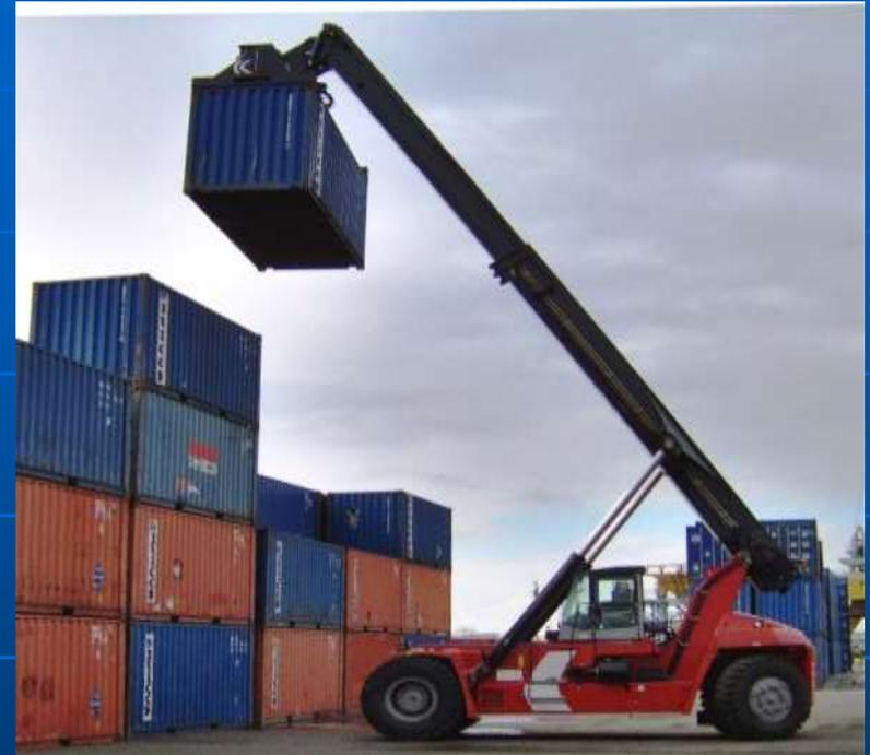
The terminal is equipped with a new latest-generation container loader model RDF450-60S5X, manufactured in Sweden by “Kalmar Industries”. The terminal allows stacking of full 42-tonne containers up to a height of 5 m.
