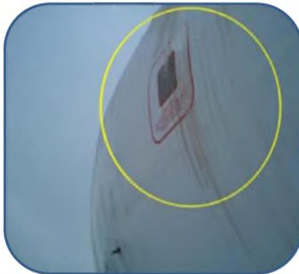
**Ice build-up in front of air data probes can lead to erroneous air data measurement.**
