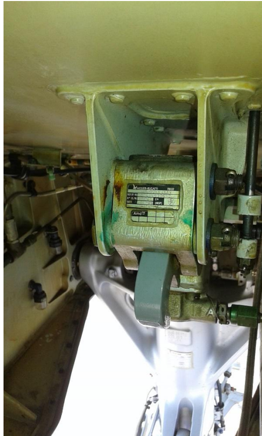
Figure 14. The failed lock of the nose L/G.
