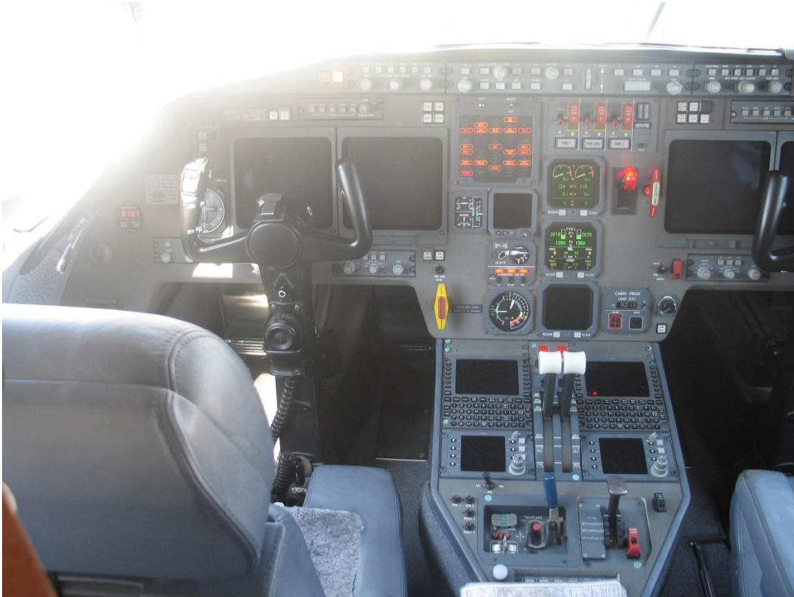
Figure 13. On the configuration panel, three red lights are illuminating.
