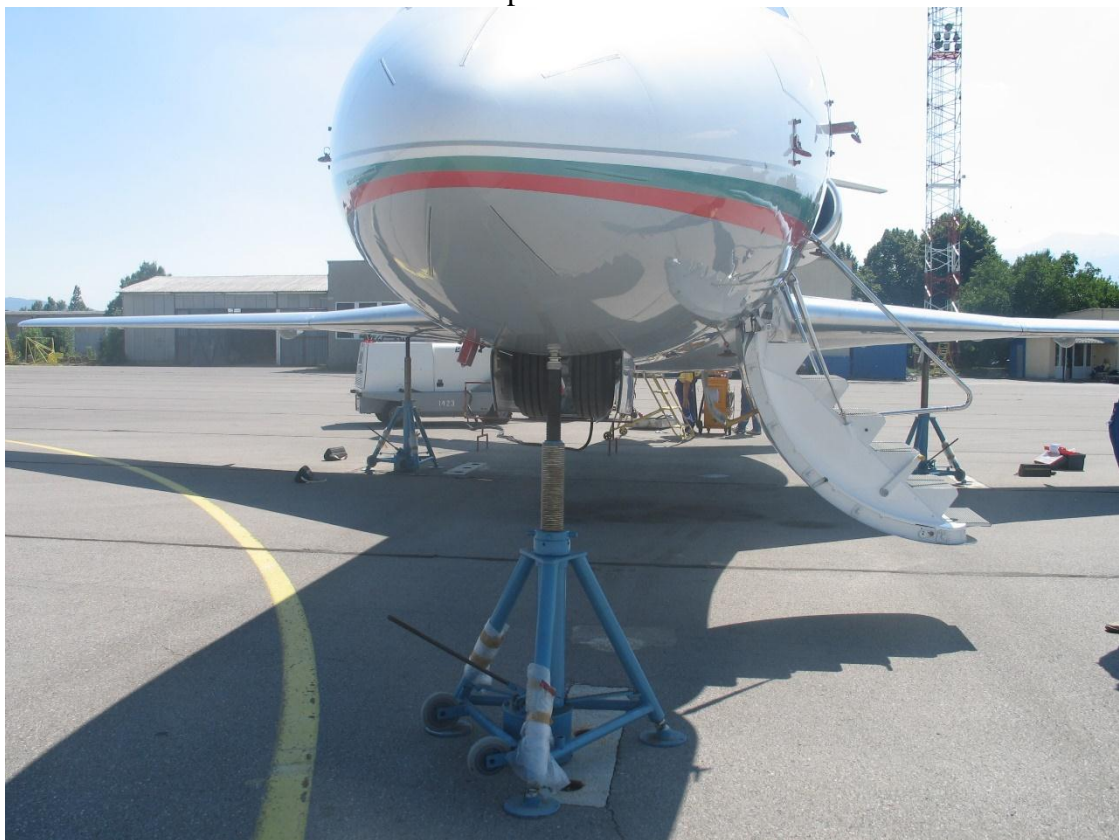
Figure 12. The lever is in “retracted” position, the nose stand is not closed in “retracted” position.
