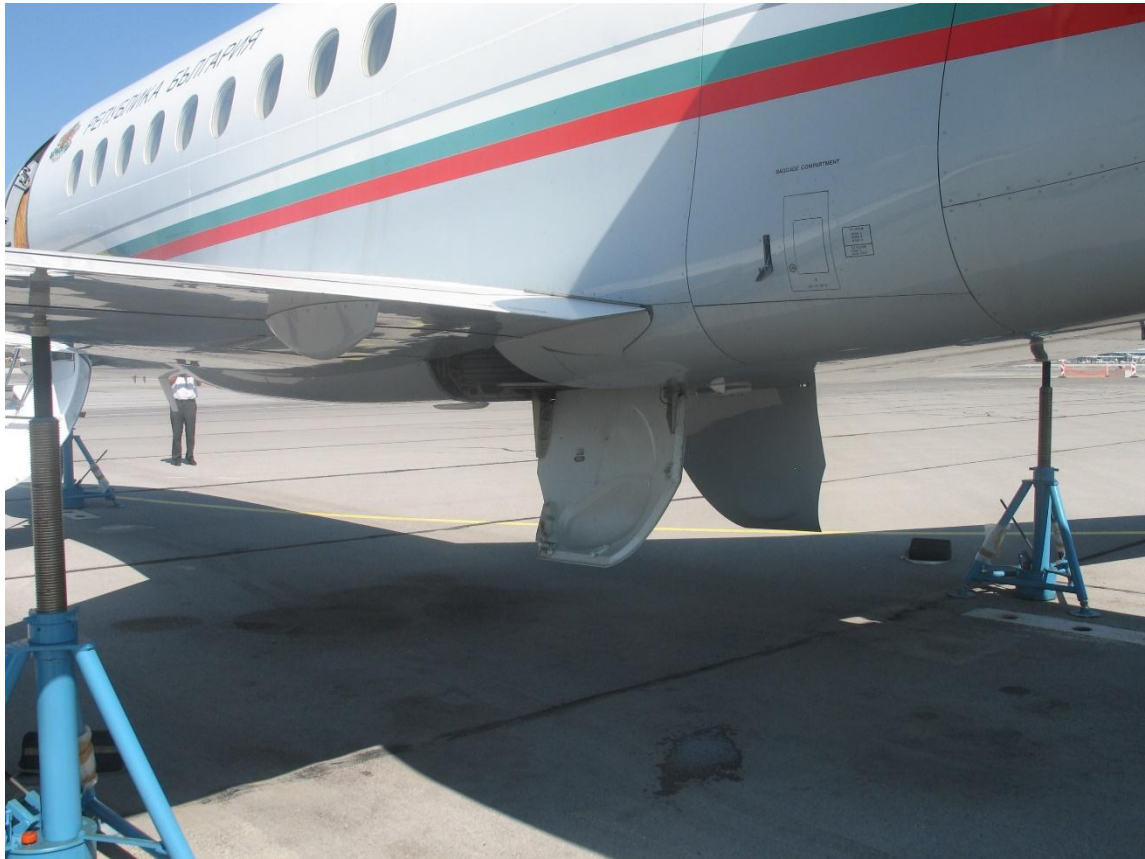
Figure 11. The lever is in “retracted” position, the doors of the main L/G remain in “down” position.
