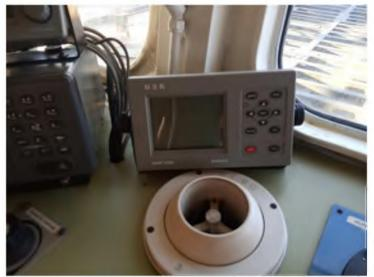
Fig. 5 — Control unit of BNWAS on the bridge
