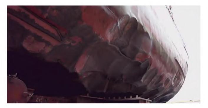
Fig. 15 Significant bends around the midship starboard side
