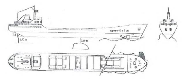
Fig. 11 — Places of contact of the hull with the bottom, at the time the vessel's grounding
