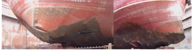
Fig. 14 Damages of the ship in the bow (port and starboard)
